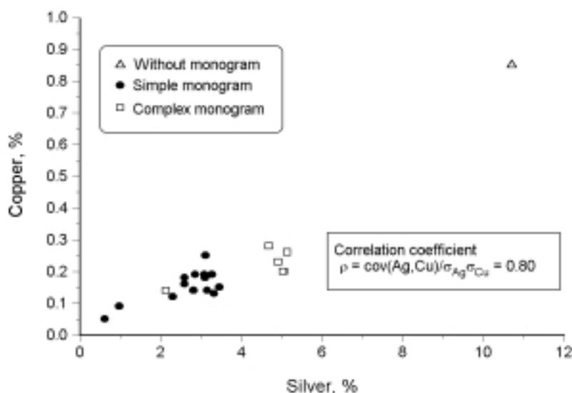
Fig. 4. Plot of the XRF results obtained for Koson coins, suggesting a correlation Cu-Ag and the existence of clusters
