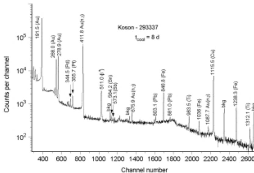
Fig. 3. Part of a gamma-spectrum of a Koson coin activated with 11 MeV protons
